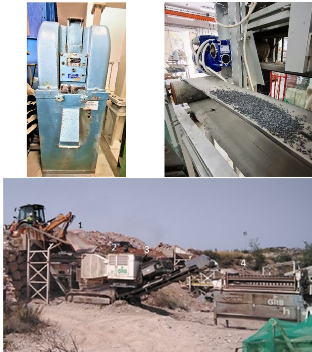
Figure 1. Top row: laboratory crushing device (left) and magnetic belt device (right). Bottom row: elements of the recycling plant, (1) hopper to receive the specimens, (2) jaw crushing machine, (3) magnetic conveyor belt, (4) sieves for the classification of the material.
